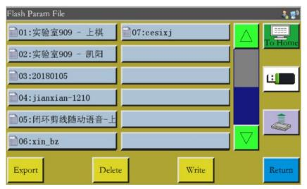
The interface displays parameters files stored in the system. Click on the file name to make it red, and then click write, when a prompt message pops up reading "In progress, please wait..." and then reading "Operation succeeded"; then, the system returns to the main interface, which means the selected parameters have taken effect. All the set values and other hidden parameters in "User parameters" and "Mechanical parameters" will be modified by this parameter file.
