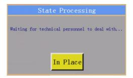
Upon the arrival of technician at the equipment, he/she can click In Place, when the machine status displayed on console reads "Waiting for solution". When Close Case is clicked after the removal of anomaly, the machine status displayed on console returns to normal.
